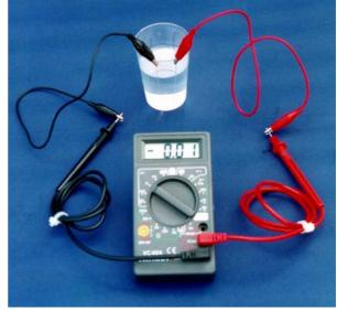
• The voltmeter is switched to the 0-20 VDC range and the battery connected to the platinum electrodes (plus to plus, minus to minus pole). One observes vigourous gas evolution at the electrodes (the chlorine gas can be smelt when close enough). The gas mixture is in principle explosive but the small quantities make the experiment harmless. The voltage of the battery is measured on the voltmeter (between 4 and 5 V).
