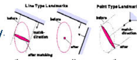
Figure 8.10: Different features can reduce the size of the robot's uncertainty ellipse in one or two directions. a, c. Walls and corners reduce uncertainty in one direction. b. Two adjacent walls at right angles reduce uncertainty in two directions. (Courtesy of [Bauer and Rosenau, 1995])
