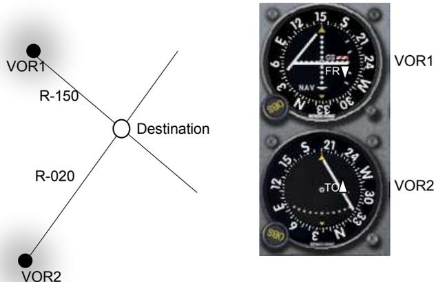
needles will center. Like before, it doesn't matter whether we put the radials at the top of the OBS or at the bottom. The results will be the same.
