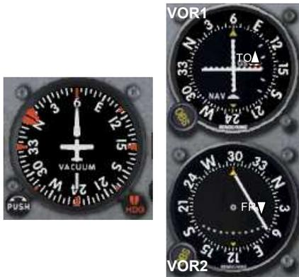
The next example highlights the most valuable use of this method. Let's say we want to fly to an intersection of two VOR radials as shown below. We tune both NAV radios and set the OBS to the required radials. Both CDI needles hit the stop. What heading should we fly to get to the intersection? Using the conventional method, this would take several minutes of OBS-twisting and mind-bending visualizations.
